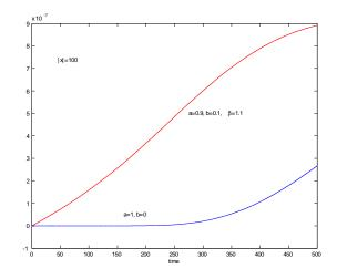
Figure 4: Comparison of the propagation time of a delta signal at (x = 0, t = 0) to a distance x = 100 for normal and mixed diffusion  $(\beta = 1.1, a = 0.9, b = 0.1)$
