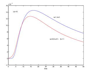
Figure 3: Comparison of the propagation time of a delta signal at (x = 0, t = 0) to a distance x = 10 for normal and mixed diffusion  $(\beta = 1.1, a = 0.9, b = 0.1)$
