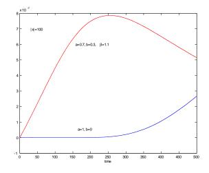
Figure 2: Comparison of the propagation time of a delta signal at (x = 0, t = 0) to a distance x = 100 for normal and mixed diffusion ( $\beta = 1.1, a = 0.7, b = 0.3$ )
